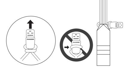
**6.** Pull the tab so that the loop tightens.
